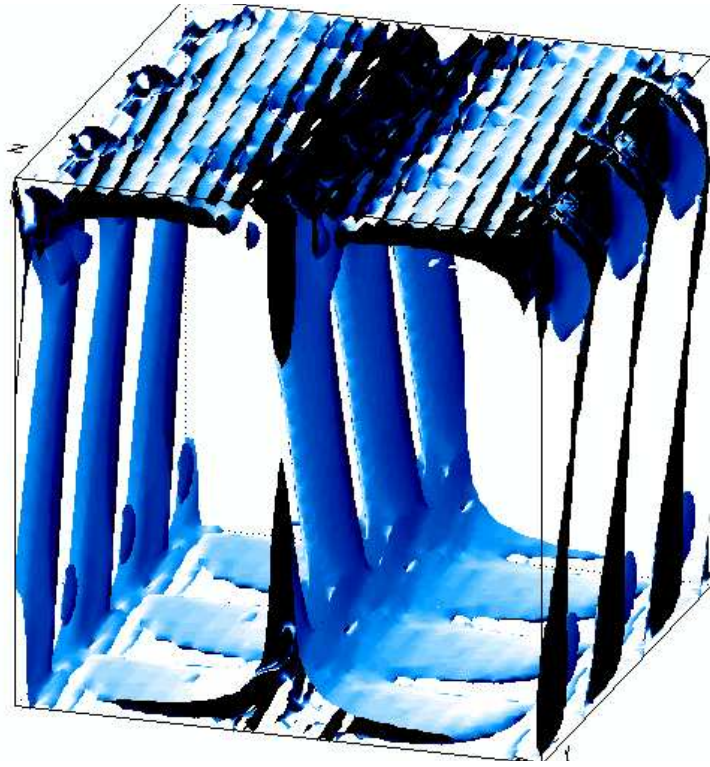
Figure 8: Growing magnetic field for the flow given by \psi , W_2 , with k = 1.5 , m = 1 and R = 2000 . An isosurface of constant magnetic field magnitude is shown in three dimensions.
